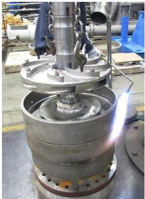
🕒 Thus, I started to disassemble the pump. Unfortunately, the casing is stuck due to corrosion. Luckily, I can find some clever tips for disassembly in a forum.
